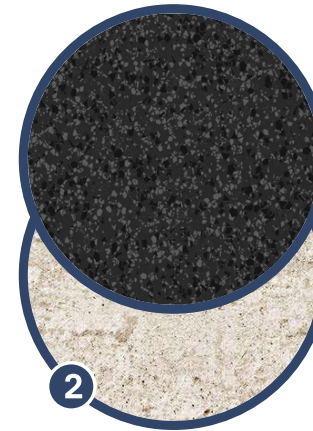
PERIMETER UP-STAND Stone or precast to match platform walls or dark terrazzo
